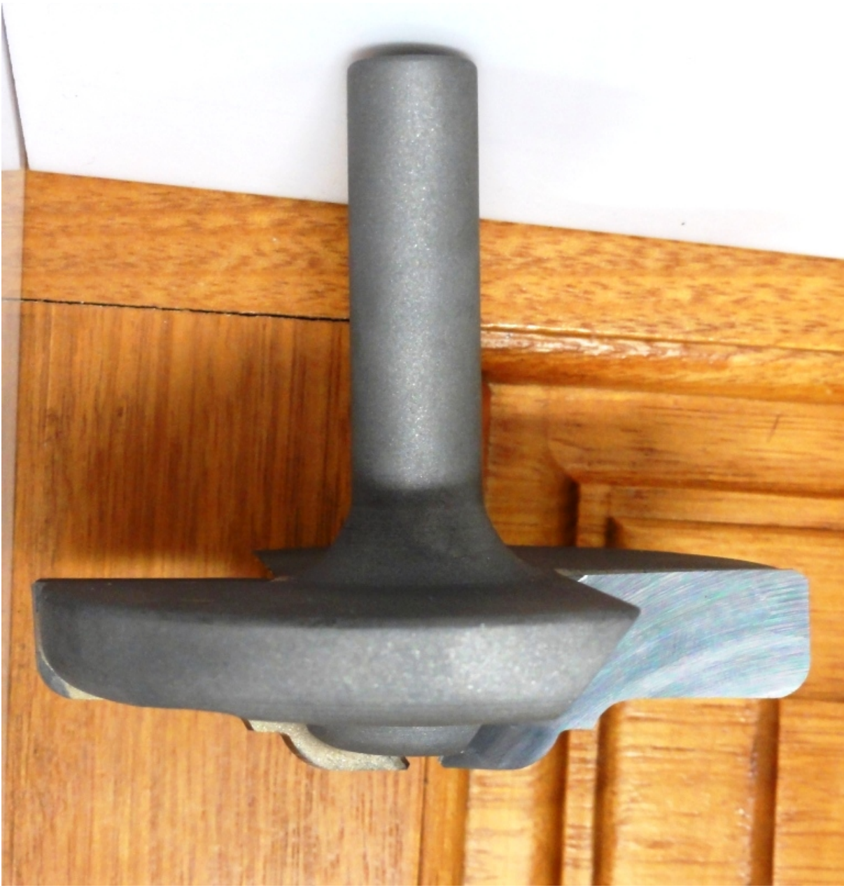
TCT Profile Router manufactured to existing door sample.
